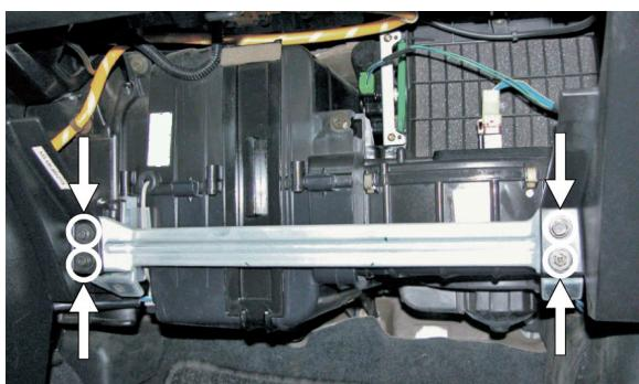
(EN) Remove the protecting device
