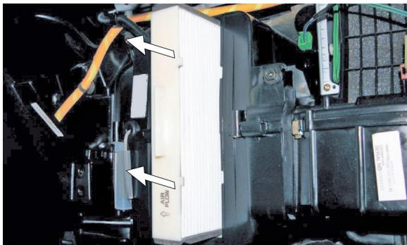
**(EN)** Take out the filter together with the frame
