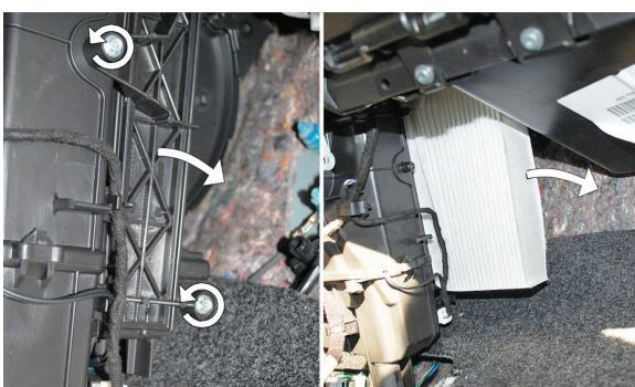
Loosen the screws and remove the cover of the filter. Gently remove the old filter, put in the new one and carry out the opposite to all the previously mentioned operations in the reversed order
